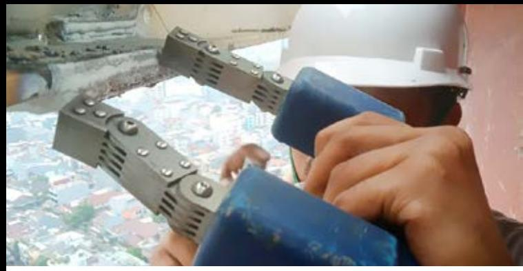
PARTICLE MAGNETIC TESTING
