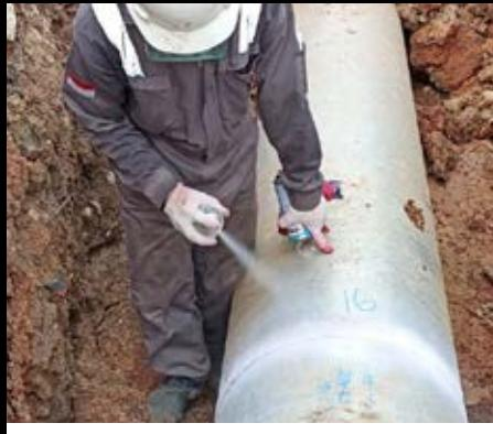
DYE PENETRANT TEST
