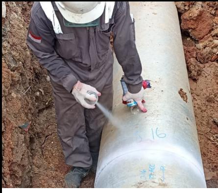
DYE PENETRANT TEST
