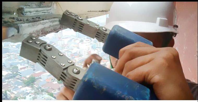
PARTICLE MAGNETIC TESTING
